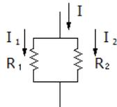
$$I_1 = I \cdot \frac{\frac{1}{R_1}}{\frac{1}{R_1} + \frac{1}{R_2}} = I \cdot \frac{R_2}{R_1 + R_2}$$
